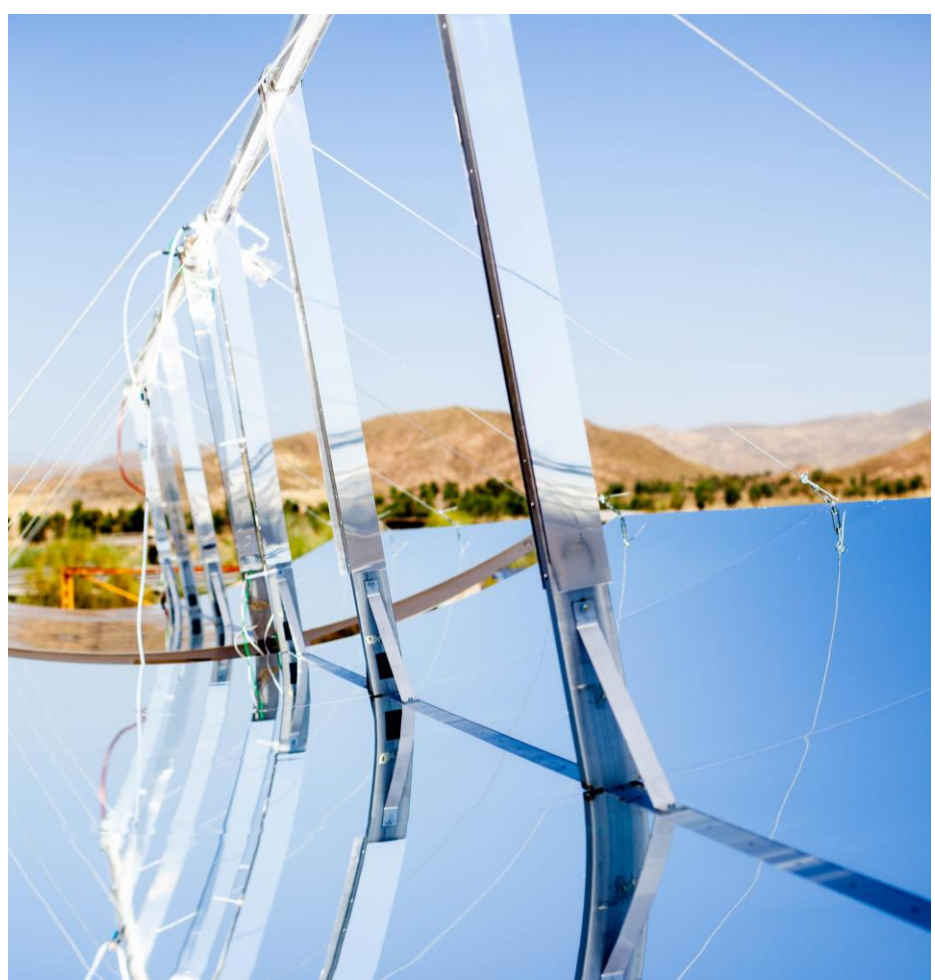
Reflector focused and tracking the sun
