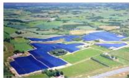
solplat's largest solar district heating plant in operation in 2015 (110 MWth) in Salzburg, Austria. Credit: Cool Energy Storage
